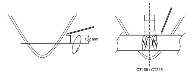
Replace the tunnel. To secure its position apply reinforced fiberglass filler to all areas, both inside and out, taking care to entirely fill the space between the hull and the tunnel. Laminate using a minimum of 8 layers of **ISOPHTALIC RESIN** alternated with mat and roving.
